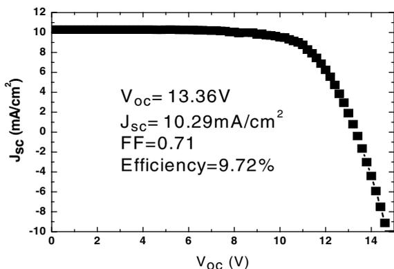
Fig. 1  $I$ - $V$  performance of an integrated 100 cm<sup>2</sup> a-Si/ $\mu$ c-Si tandem cell.
