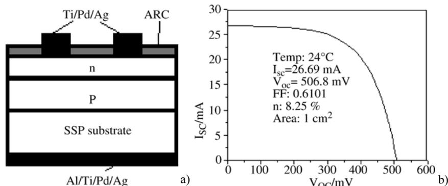
Fig. 4 Poly-Si film solar cell on SSP ribbon substrate, (a) cell structure, (b)  $I$ - $V$  curve of the solar cell.
