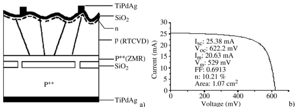
**Fig. 3** Poly-Si film solar cell on modeling ceramic substrate (nonactive Si substrate covered by  $\text{SiO}_2$  layer), (a) solar cell structure, (b)  $I$ - $V$  curve of the cell.
