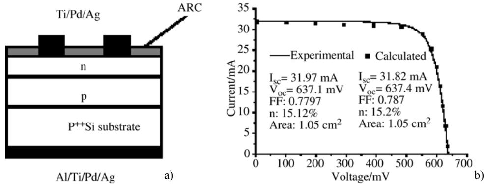
**Fig. 2** Poly-Si film solar cell on nonactive silicon substrate, (a) cell structure, (b)  $I$ - $V$  performance of the cell.
